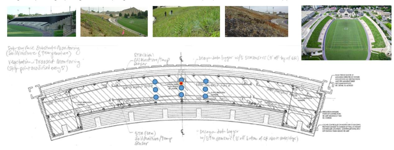
On June 20, 2016 we installed 9 Decagon 5TM Soil Moisture/Temperature sensors 3 inches below the surface to better understand changing conditions on the West and East MS Green Roofs; we plan to compare our initial data with plant coverage (using UAS aerials) and species richness (using transects) over a multi-year period.
