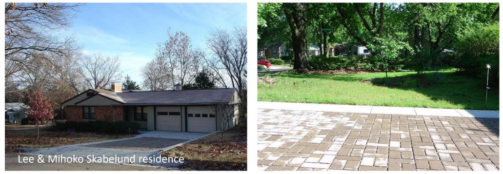
Stormwater entered our basement too many times, so I designed and had implemented a permeable driveway, vegetated swales, and rain gardens with disconnected downspouts moving water onto our lawn (warm season grass that needs minimal water & mowing).
