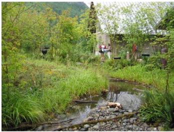
Roof water is collected in carved stone basins, then drains into a grated channel before cascading over a five-foot stone-faced retaining wall. The learning lab and auditorium buildings expand onto the courtyard, with tile artifacts historically manufactured in the watershed. Surrounding forest and meadows are pulled into the courtyard and onto building roofs.
